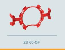
Application tip: OBO Quick-Fix and the flush-mounted box are inserted together in a hole with a diameter of 82 mm. The straps then bend, fixing the flush-mounted box. The ends of the straps have nail holes, for additional fastening of the Quick-Fix quick fixer on the wall with nails.
